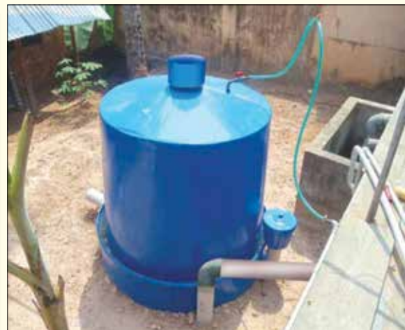
Figure 3.17 Portable Household Biogas Plant
